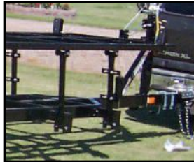
Sturdy Cross Brace With Nylon Bushings (Standard Models Only)
