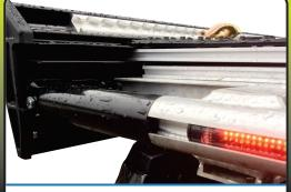
Supertrac runs the length of the side extrusion & c/w 4 tie downs. Supertrac slides directly into the extrusion to give more deck space and secure the Superglide
