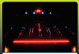
New LED tail, signal & reverse lights embedded in rear loading bar extrusion. LED bullet lights on headache rack and under the deck
